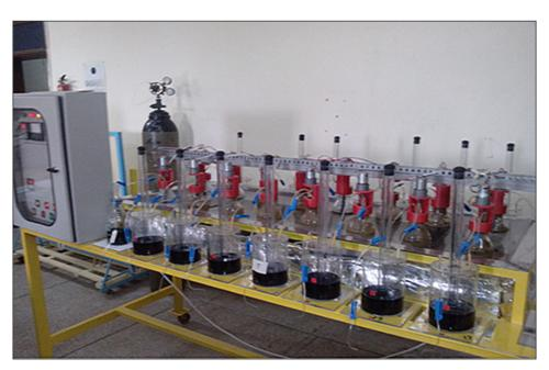
Figure 1. Semi-automatic metahne potential test system
